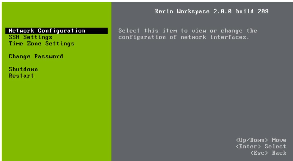
Figure 1 Console — network configuration
