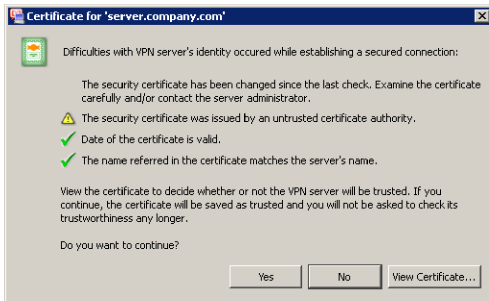
Figure 2.6 A dialog informing about detected problems with the VPN server's certificate
