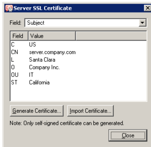
Figure 12.2 Kerio Control's web interface SSL certificate
